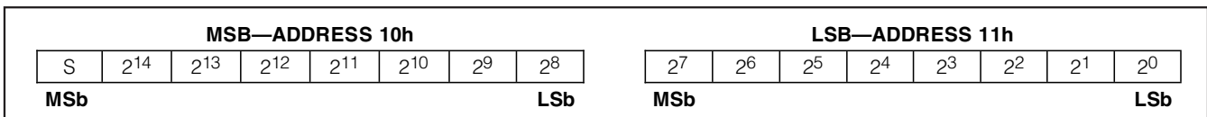
Figure 2. Current Accumulator Register Format
